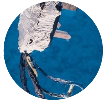
Chew damage to plug
