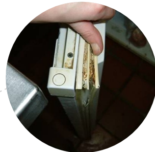
Seal of refrigerator door
